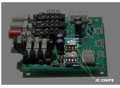
There are (2) IC chips used in the MINI-IO Module kit.
