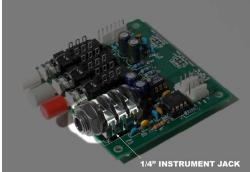
Plug your electric guitar or bass into the front 1/4" jack. Press the Mic/instrument select switch (RED) to switch between mic inputs and Instrument input.
