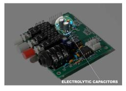
Electrolytic capacitors are cylindrical in construction. Unlike ceramic capacitors, electrolytic capacitors USUALLY/MOSTLY have polarity. One side is marked with the (-) sign, also called the cathode, or negative side.
