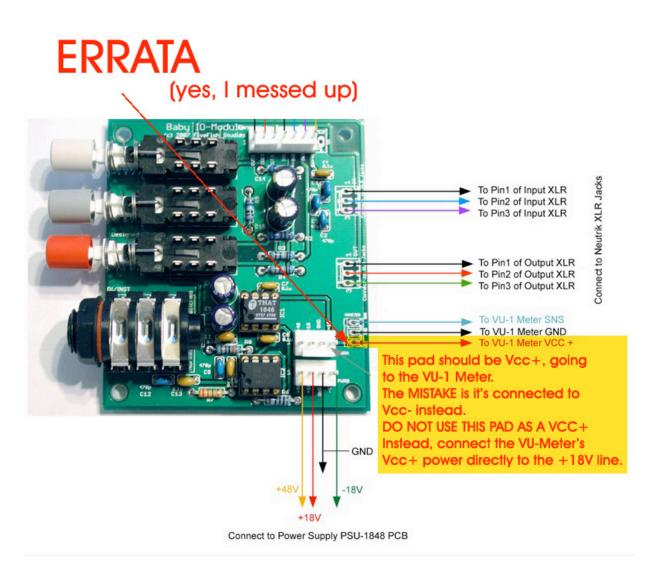
Please connect the Vcc+ of the VU meter directly to the Power Supply's +18V instead.
