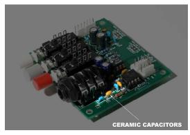
Capacitor parts are therefore rated with their capacitance (in microfarads, uf) and voltage... specified like this: 0.1uf 100V
